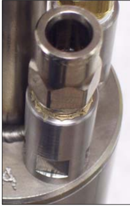
Air Inlet Push-To-Connect 1/4 in O.D. Nylon Tubing
