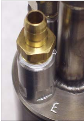
Exhaust Hose Barb 3/8 in O.D. x 1/4 in I.D. Nylon Tube.
