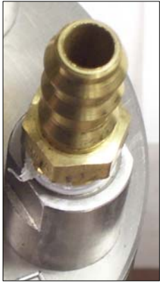
Exhaust Hose Barb 3/8 in I.D. Buna-N Hose
