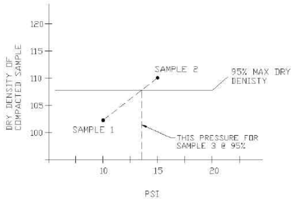
FIGURE 1: DRY DENSITY VS. PRESSURE
