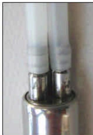
The barb fitting on the top of the TR-035 and TR-037 stainless steel pumps are marked with an "A" for the air line. If Durham-Geo bonded tubing is used (Teflon<sup>®</sup> lined polyethylene and polyethylene), the rougher surfaced Teflon<sup>®</sup> lined tube should be connected to the unmarked fitting and the smooth surfaced polyethylene tube to the "A" fitting. Note: You can see the Teflon lining
