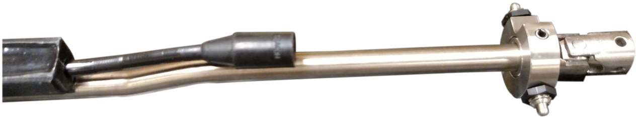
Figure 4: GeoFlex bottom node (female connector and universal joint)
