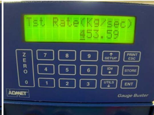
Input test rate & press "Ent"
