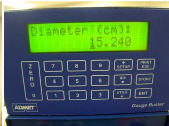
For Cyl type, input diameter, & press "Ent"
