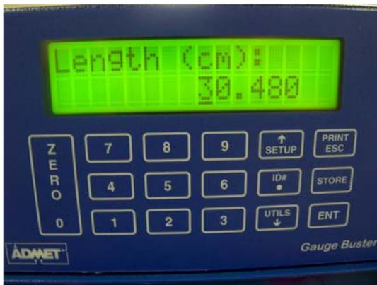
For Cyl type, input length, & press "Ent"
