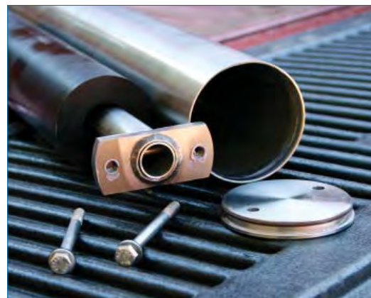
Top-loading pump, TR-974, disassembled.
