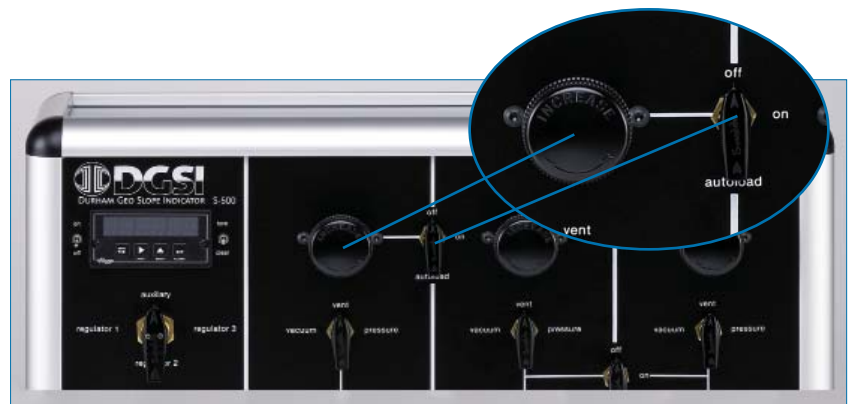
Close-up of the differential regulator (E-656) which is unique to the DGSi permeability / triaxial panel.
