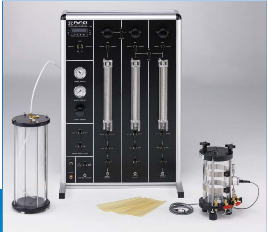
S-500 Master panel for one test cell. Shown with membranes, permeability cell and deairing tank (sold separately).
