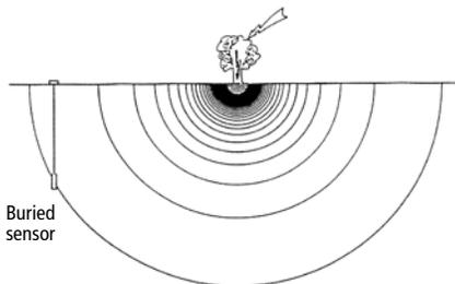
In the drawing above, the cable to the sensor cuts across part of one level, so there is about a 10 to 20 kV voltage gradient between the surface and the sensor.
