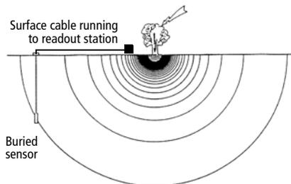
One way to eliminate this gradient is to run a ground wire parallel to the horizontal signal cable and connect it to the grounding wire in the borehole. This is generally not cost-effective unless an existing grounding grid can be used.
