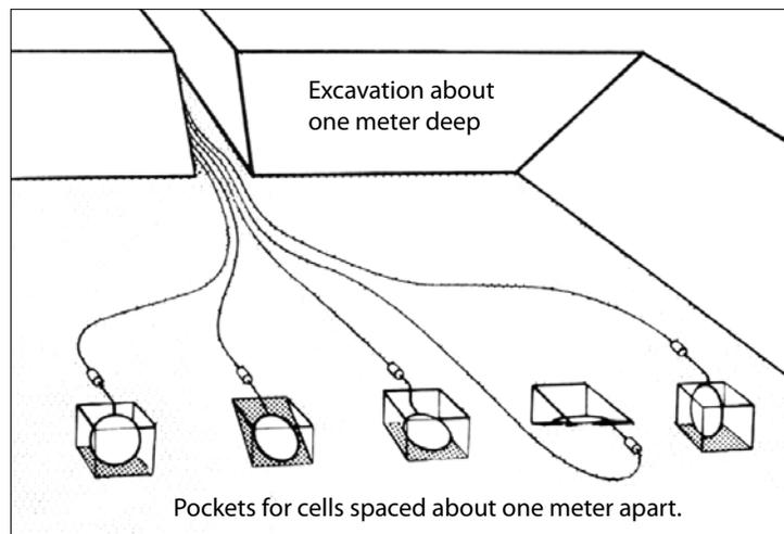
1. Make a one-meter deep excavation in the fill. The excavation should be large enough to accommodate all of the pressure cells, spaced at least one meter apart. The floor of the excavation should be levelled and compacted. Also excavate a trench for cables.
