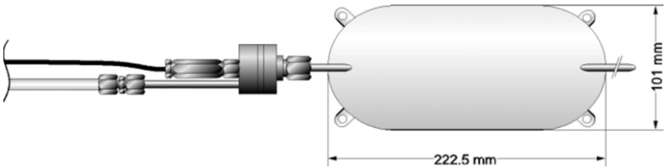
Fig. 3 INTERFELS Tangential Total Pressure Cell with Membrane Switch, Mounting Eyes and Post-Tensioning Tube ((also available: VW Pressure Transducer)
