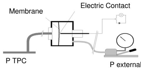
*Measuring Principle of INTERFELS Membrane Switch*
