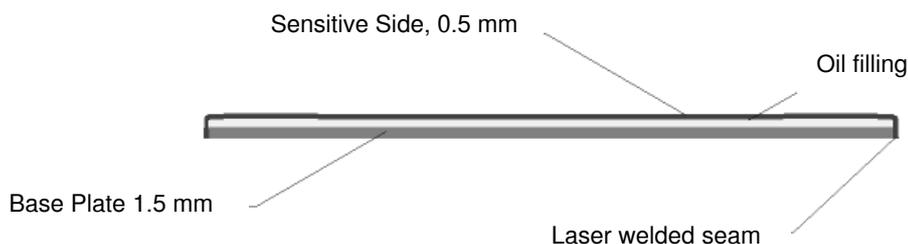
Fig. 1 Cross Section of an INTERFELS TPC
