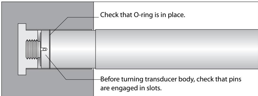
6. Secure transducer body and cable for concreting. Tie body to nearby rebar and add protection if possible. Find a safe route for signal cable. Devise protection for cable where necessary. Route cables away from sources of electrical noise, such as motors or AC power lines.
