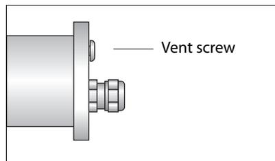
9. Connect readout and take reading to verify that jointmeter is working. Note serial number of jointmeter, too.
