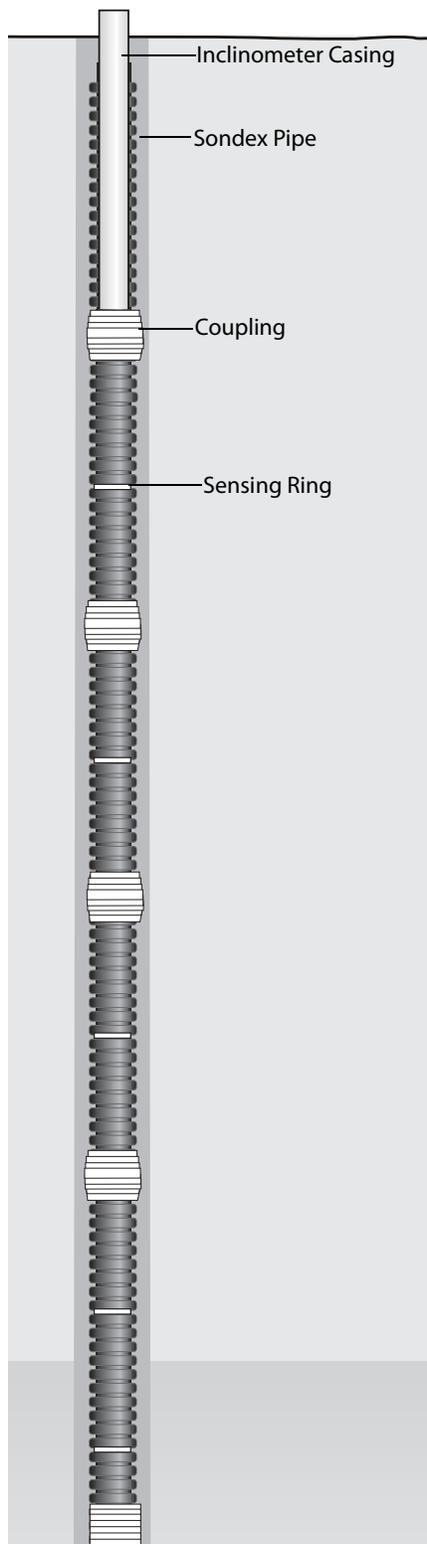
In a typical sondex installation, flush-joint, inclinometer casing is installed inside corrugated sondex pipe. The bottom section of corrugated pipe is attached to the casing. The remaining pipe is left unattached to move with settlement/heave.
