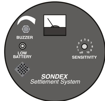
**Buzzer.** Buzzer alerts operator when probe is in the vicinity of a sensing ring. Meter response is inhibited while buzzer sounds. Buzzer is factory set and should not be adjusted.
