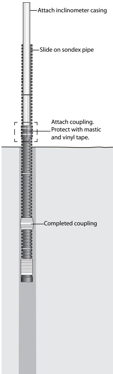
Once the bottom sections have been attached continue to add sections of inclinometer casing and corrugated pipe. Attach the corrugated pipe using sondex couplings.
