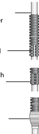
You may want to attach a grout hose to the bottom section as it may be difficult to work a grout hose between the corrugated pipe and the borehole wall.
