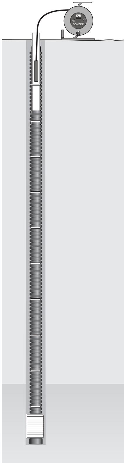
The Sondex Settlement system is used with inclinometer casing to measure settlement and heave associated with excavation, construction, backfill, or tunneling operations.
