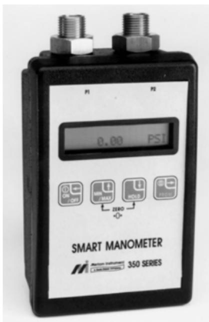
Meriam Instrument's 350 Smart Manometer is a microprocessor based pressure sensing device that can be used to directly measure pressure. Differential pressure units (clean dry gases only) can also measure flow when used with a square root type primary flow element. Models are available to measure gauge, absolute, differential and vacuum pressure in ranges from 20" w.c. to 2000 PSIG. Pressure can be displayed in a variety of user selectable engineering units.
