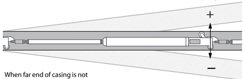
When far end of casing is not stable, displacements are referenced to the near end.
