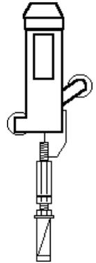
Swivel clamp: Locks the swivel on the bottom wheel assembly.
