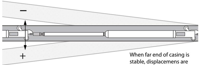
A positive displacement value indicates movement in the direction of the fixed wheels.
