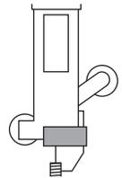
Tubing clamp: Connects the sensor to the gauge tubing of another sensor. Supplied with the sensor.
