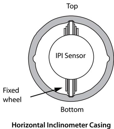
Horizontal Inclinometer Casing
