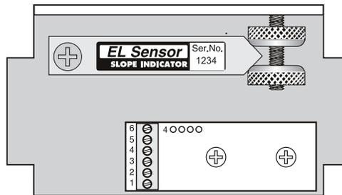
**About Zeroing** Zeroing is the process of adjusting the sensor so that its output is as close as possible to zero. Since the sensor is very sensitive to even small movements, you must connect signal cable to it before you adjust the sensor. Otherwise, you may have to re-zero the sensor after the signal cable has been attached.
