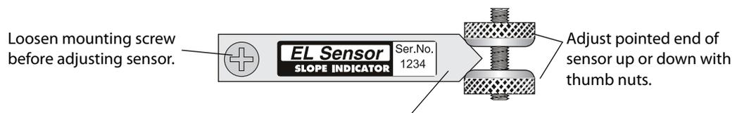
If readings are negative, pointed end of sensor should be moved upward.
