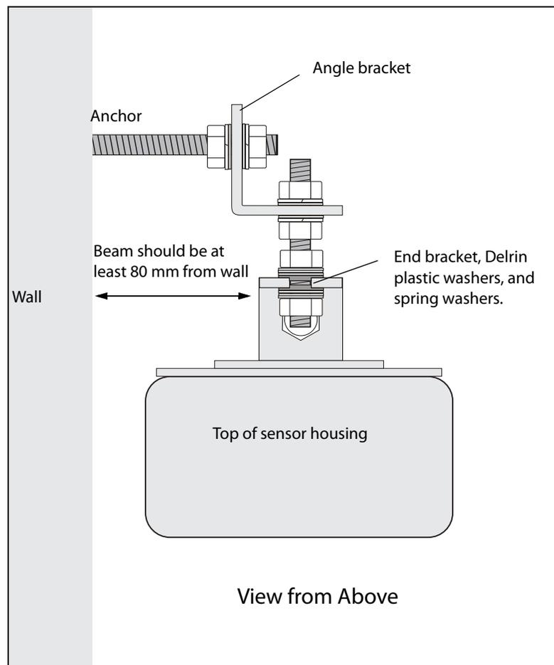
4. Viewed from the front, beam should be near vertical. Viewed from the side, the beam should be roughly parallel with the wall.
