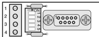
Standard terminal board has 4 terminals. Other notable features are a DB9 connector and a bank of switches.
