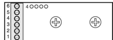
SC terminal board has 6 terminals. The only other notable feature is the row of four pins at the top of the board.
