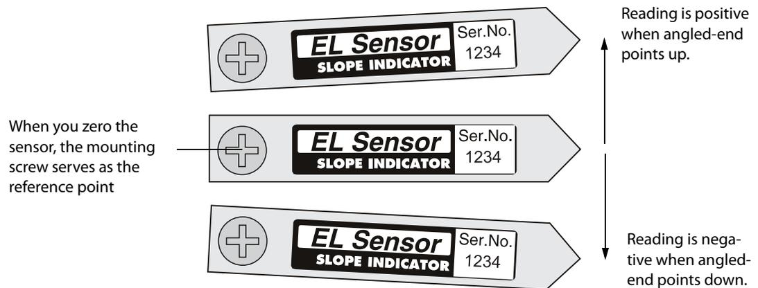
Note that the relation between up and positive and down and negative would be reversed if you held the angled-end of the sensor and moved the screw end up or down.
