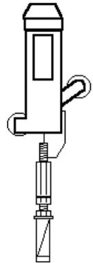
**Swivel clamp:** Locks the swivel on the bottom wheel assembly.
