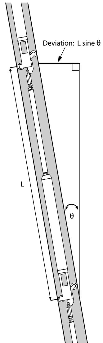
**Displacement** Displacement, the distance the casing has moved, is calculated by subtracting the initial deviation from the current deviation. The displacement value will be negative or positive. This indicates the direction of movement, as shown below.
