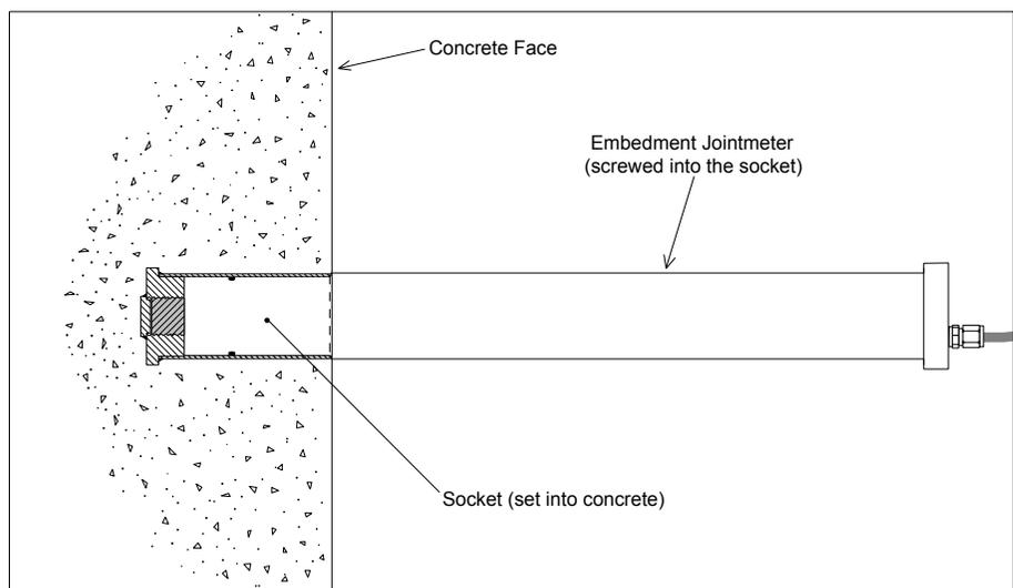
Figure 3 - Embedment Jointmeter Installation
