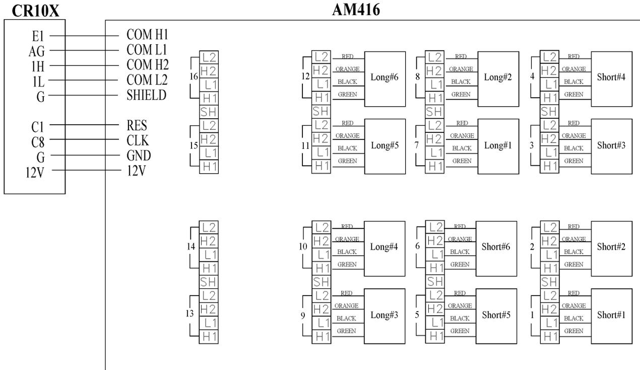
Note: For each sensor, drain wire for screen or shield should be connected to L1 terminal on AM416.
