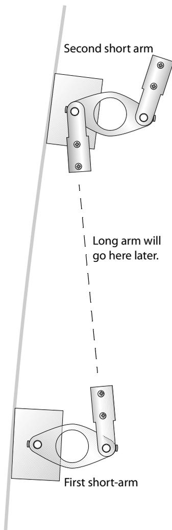
1. Start at the bottom pivot pin on the left side. Avoid working from both sides at once.
