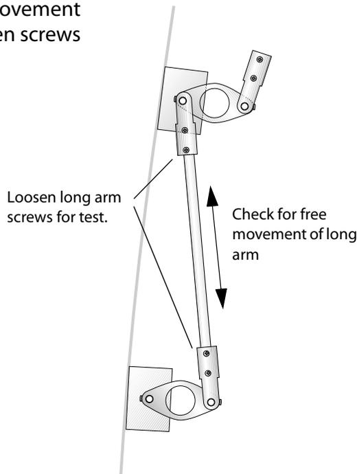
Follow the procedure below to check movement of each arm. Work from left to right.
