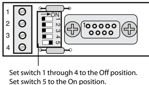
2. Connect the EL zeroing device or DataMate MP to the DB9 socket on sensor board and switch on.
