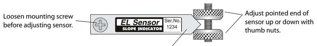
If readings are negative, pointed end of sensor should be moved upward.
