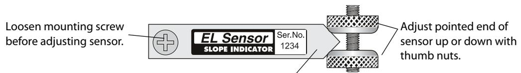
If readings are negative, pointed end of sensor should be moved upward.
