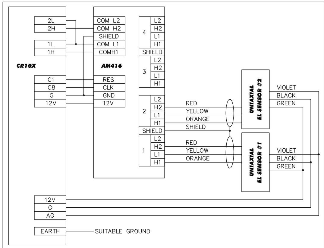
Wiring Diagram 4 Connecting biaxial sensors to an AM416 multiplexer
