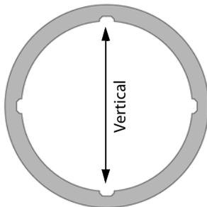
In horizontal installations, one pair of casing grooves must be aligned to vertical.
