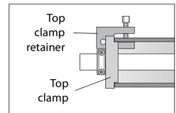
3. In horizontal installations, the sensors normally must be pushed into the casing. This puts the mechanical linkage of the sensors into compression. If possible, put the linkage into tension, but pushing the sensors deeper into the casing and then pulling them back into position.
