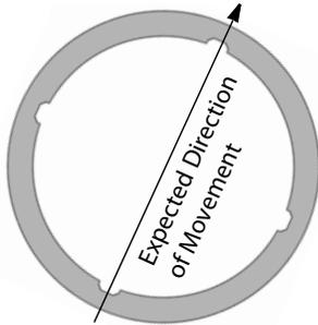
In vertical installations, one pair of casing grooves should be aligned with the expected direction of movement.
