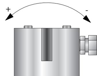
Side view. Tiltmeter monitors tilt in the plane of the arrows.
