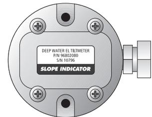
Top view, looking down at the tiltmeter. Surface with label must be horizontal.
