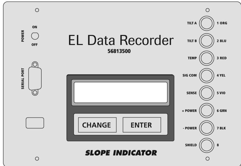
**Power Switch** The power switch turns power on and off. The Recorder goes into standby mode if no key is pressed for a period of time. To restore full power, press any key, or switch the Recorder off and on. When you are finished taking readings, always switch the recorder off.
