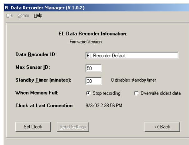
**Data Recorder ID** Enter an identifier for the Recorder. This ID does not appear in the data file.
