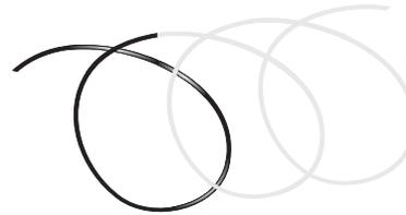
2. Twist cable backwards to make a second loop as shown in drawing.
