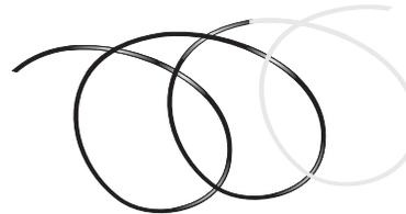
3. Continue coiling cable with alternating loops as in step 1 and 2 above.
