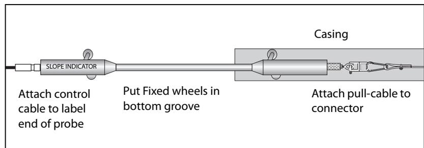
Inserting the Probe for the 1st Pass
