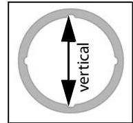
**Probe**    **Fixed Wheels:** The fixed wheels (as opposed to the sprung wheels) of the probe are kept in the bottom groove of the casing during both passes of the survey.
