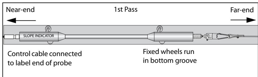
**Second Pass:** At the end of the first pass, the probe is reversed end for end and control cable and pull cable are reconnected. The probe is then reinserted in the casing, fixed wheels still in the bottom groove.
