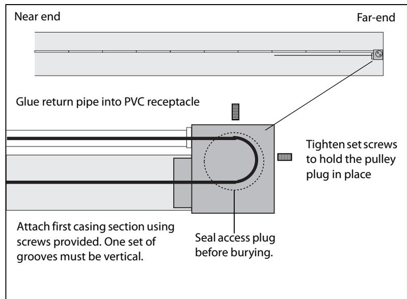
3. Assemble casing, starting at the far-end. Orient casing so one set of grooves is vertical. Pull stainless steel cable through as you add casing sections. If you are using a dead-end pulley, attach the first section of casing using the screws provided.
