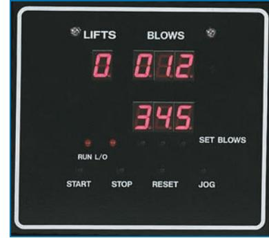
Display shows the number of lifts and blow counts (per layer). Blows can be pre-set and automatically stop the machine. Hammer jogging button and auto parking for hammer are standard.
