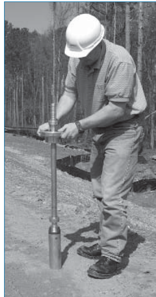
2 - Driving the Sampler Tube. The operator is about to release the 15-lb mass.
