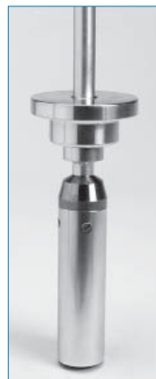
S-20037 w/ 3 x 10-in Sampler (Shelby) Tube
