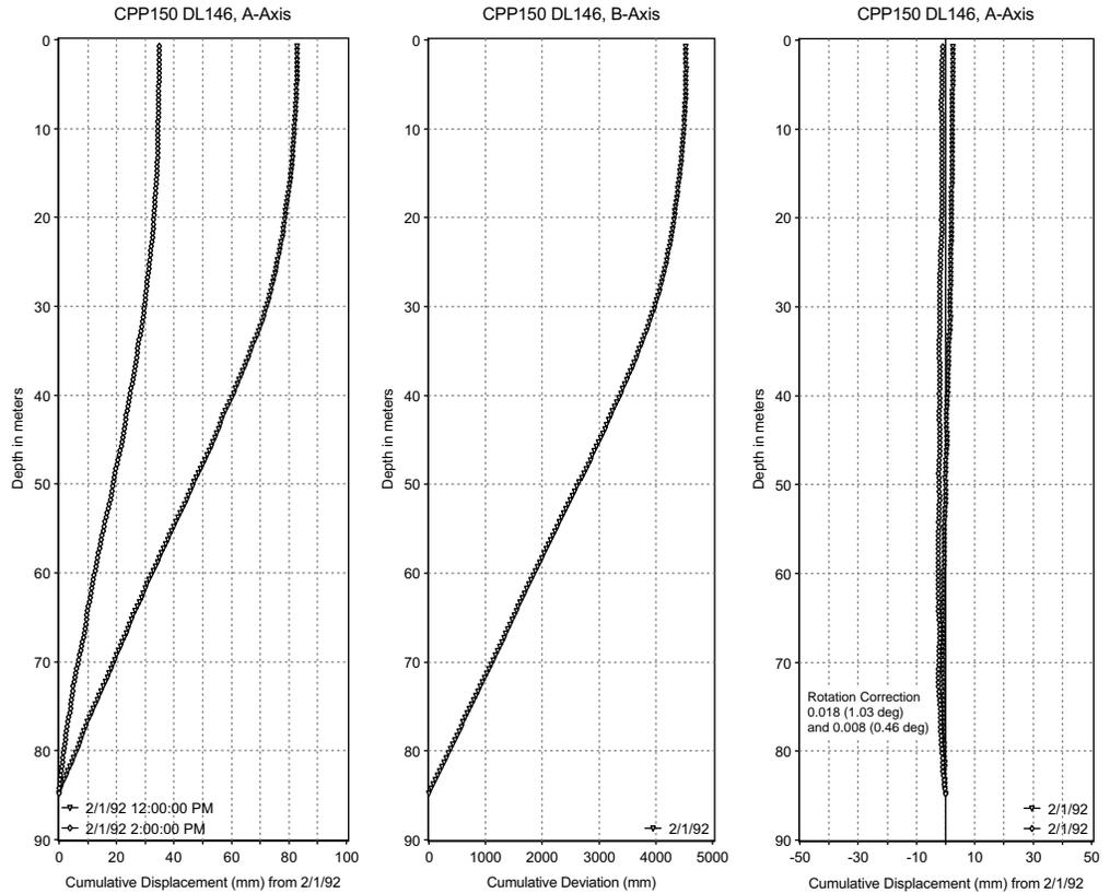
Cumulative Displacement Plot, A-Axis, Before Correction
