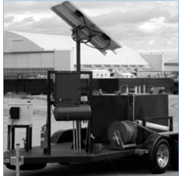
SolarNAPL, custom mounted on dual axle trailer (TR-51660).
